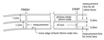
Figure TR 14 (Rule 160) - Track Measurements (Infield View)
