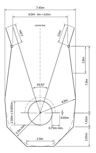
Figure (b) TR37 (Rule 192) - Cage for Hammer and Discus Throw with concentric circles (Discus Throw configuration, with cage dimensions to netting)
