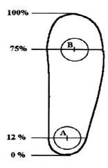
Figure (b) TR5 (Rule 143) - Location for measurement of the centre of the forefoot and heel
